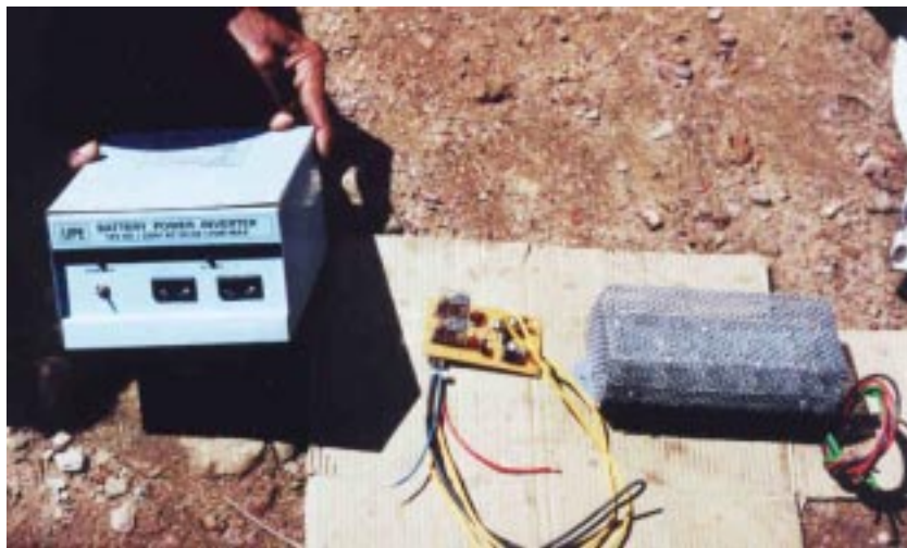
Photo 7: Left to right: Inverter, charge control circuit, and dump load, in Sri Lanka. (Simon Dunnett,)
