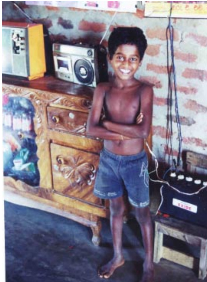
Photo 2: a 12 volt car battery used for radio and TV in Sri Lanka (Simon Dunnett,)
