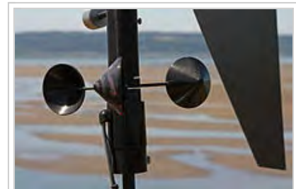
Cup-type anemometer with vertical axis, a sensor on a remote meteorological station
