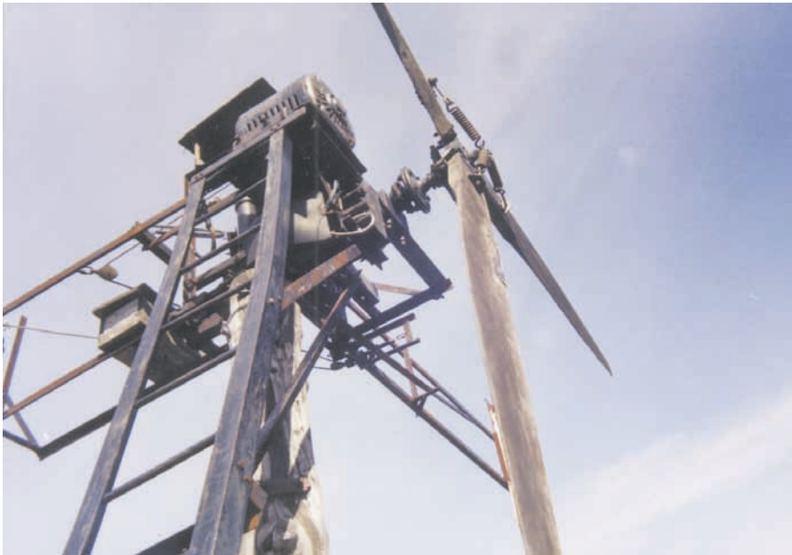
The top ladder section is affixed to the genny and yaws with it.
