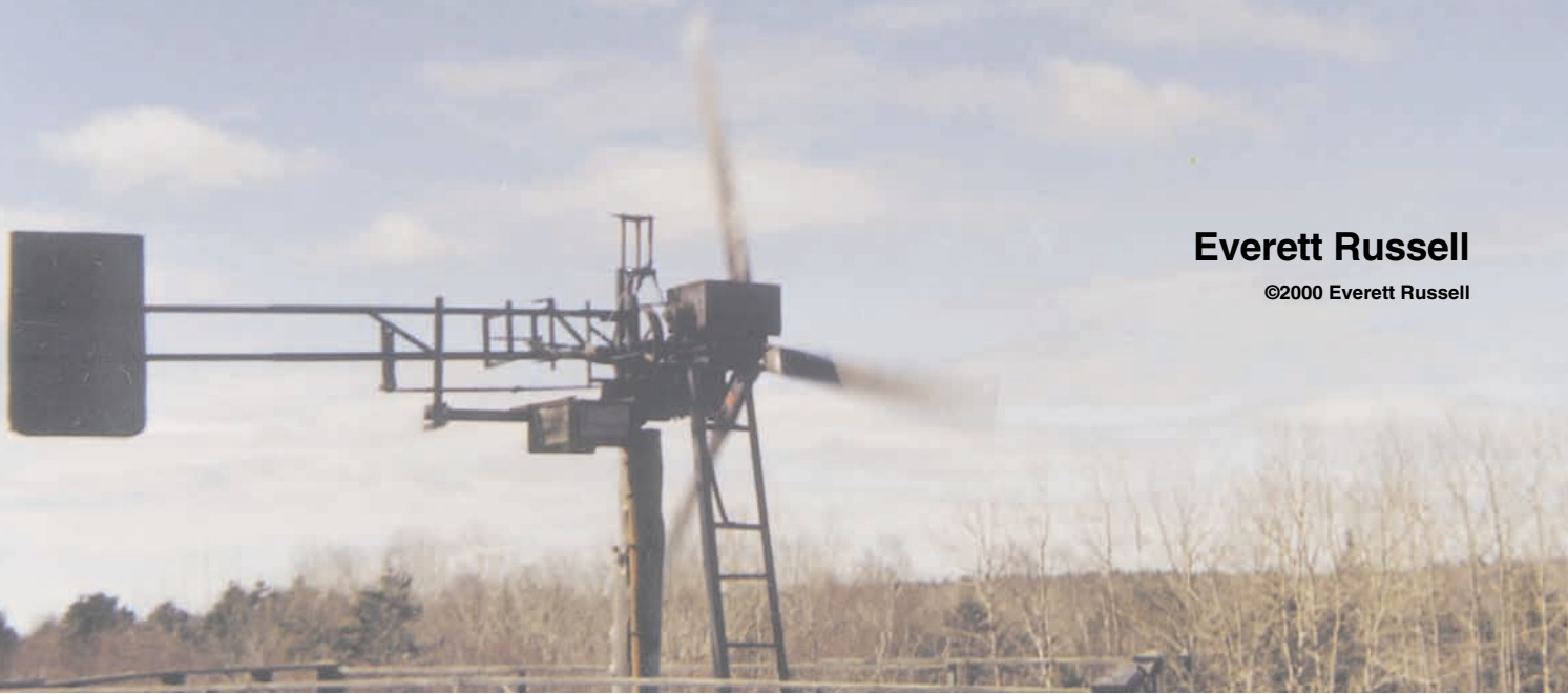
One of Everett Russell's two home-built wind generators with a 14 foot rotor diameter.
