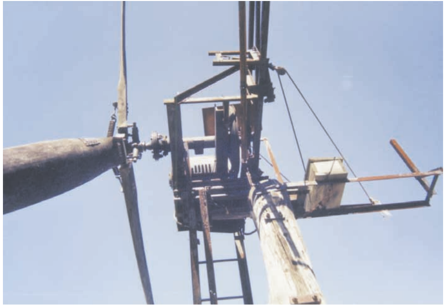
Looking up from below: the genny's tail structure is folded to the side.
