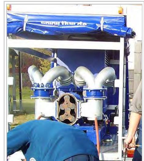
Lobe pump (5m<sup>3</sup>/min or 1886 barrel/h) of THW
