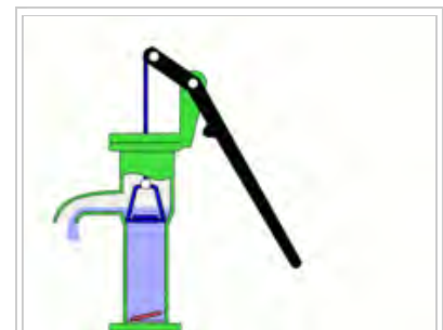
Cross section and details of a pitcher pump
