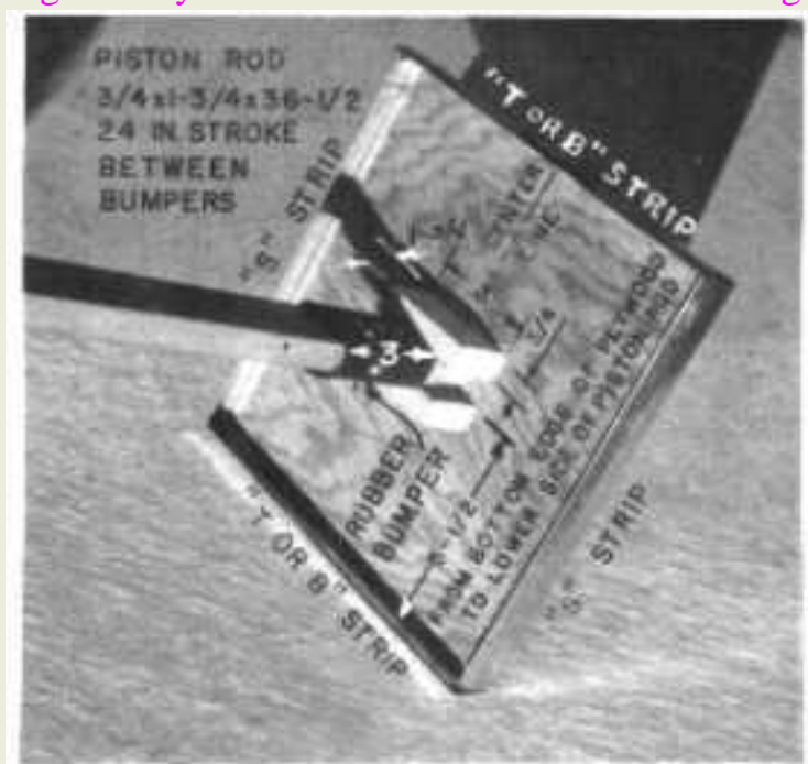
Fig. 14. Plywood Piston with Sheetmetal Sealing Strips Attached.
