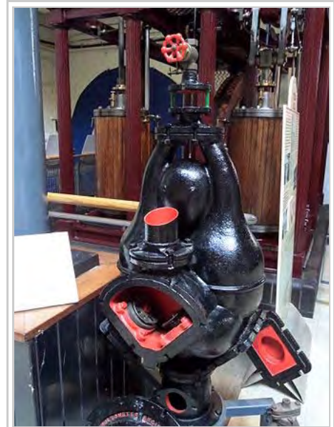
Pulsometer pump at the London Museum of Water & Steam
