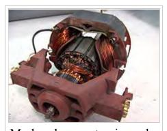
Modern low-cost universal motor, from a vacuum cleaner. Field windings are copper colored, toward the back, on both sides. The rotor's laminated core is gray metallic, with darker slots for winding the coils. The commutator (partly hidden toward the front) has become dark from use. The large brown molded-plastic piece in the foreground supports the brush guides and brushes (both sides), as well as the front motor bearing.
