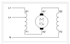
Universal motors' field coils are series wound with the rotor coils and commutator
