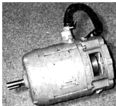
FIGURE 12-14 Typical DC shunt motor. These motors are available in a variety of sizes. This motor is a 1 hp (approximately 8 in. tall).
