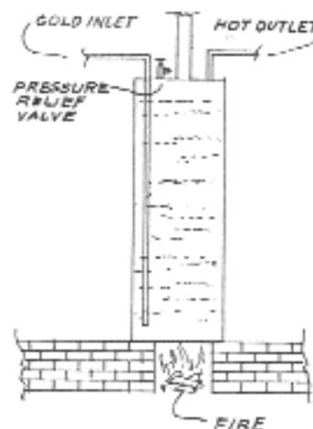
Figure 2. Water tank heated directly by fire.
