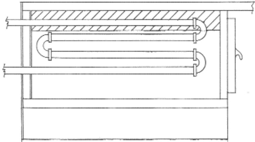
Figure 3. Cast iron pipe arrangement inside a firebox.
