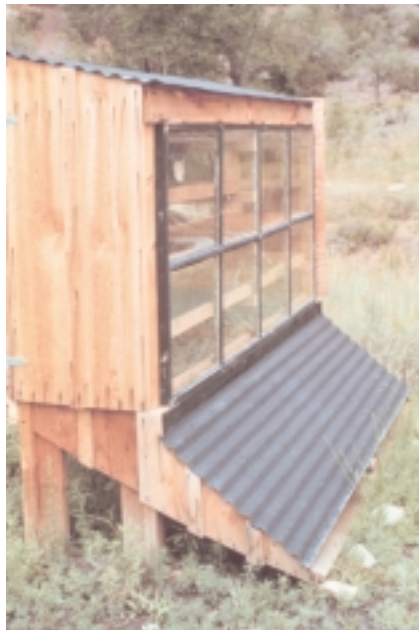
A solar-powered food dehydrator lessens the need for refrigeration.
