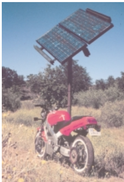
This electric motorcycle is recharged daily from two solar modules.
