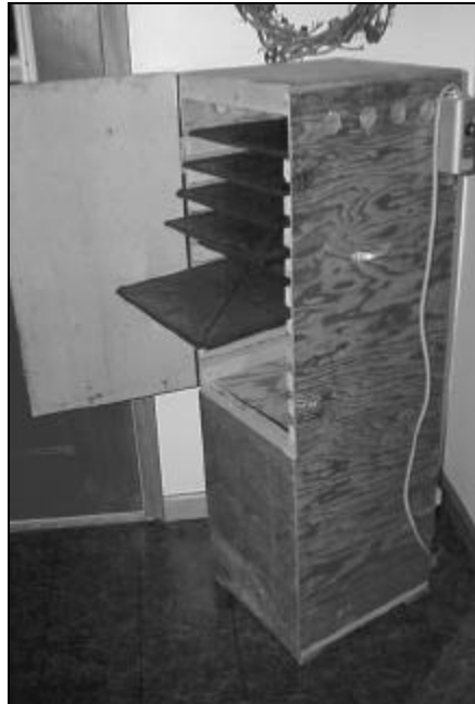
Left: The dryer cabinet and the polycarbonate trays. Right: The 600-watt ceramic heat coil screws into an ordinary porcelain lamp base.
