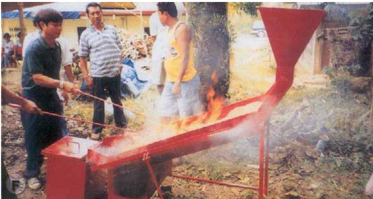
f. The metal plate carbonizer is a simple low-cost machine capable of carbonizing not only sawdust and rice hull but also coconut coir dust and other carbonaceous fine materials.
