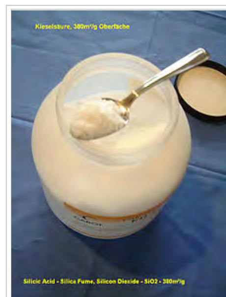
Manufactured silica fume at maximum surface area of 380 m 2 /g
